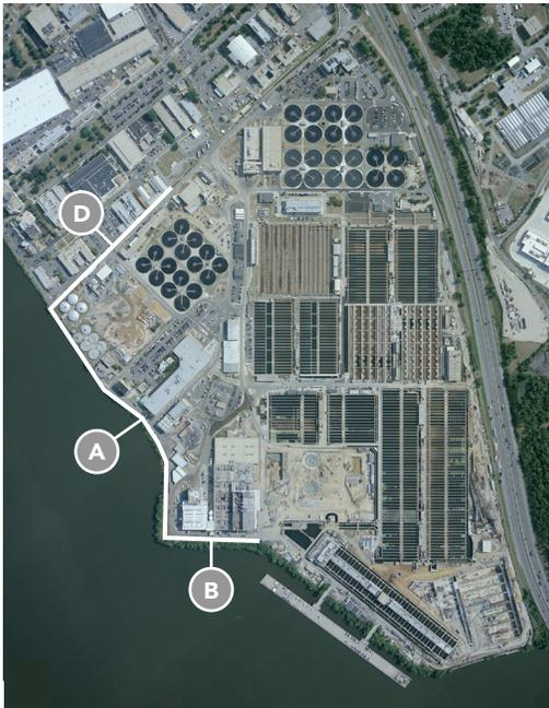
Conceptual alignment of floodwall segments A, B, and D
