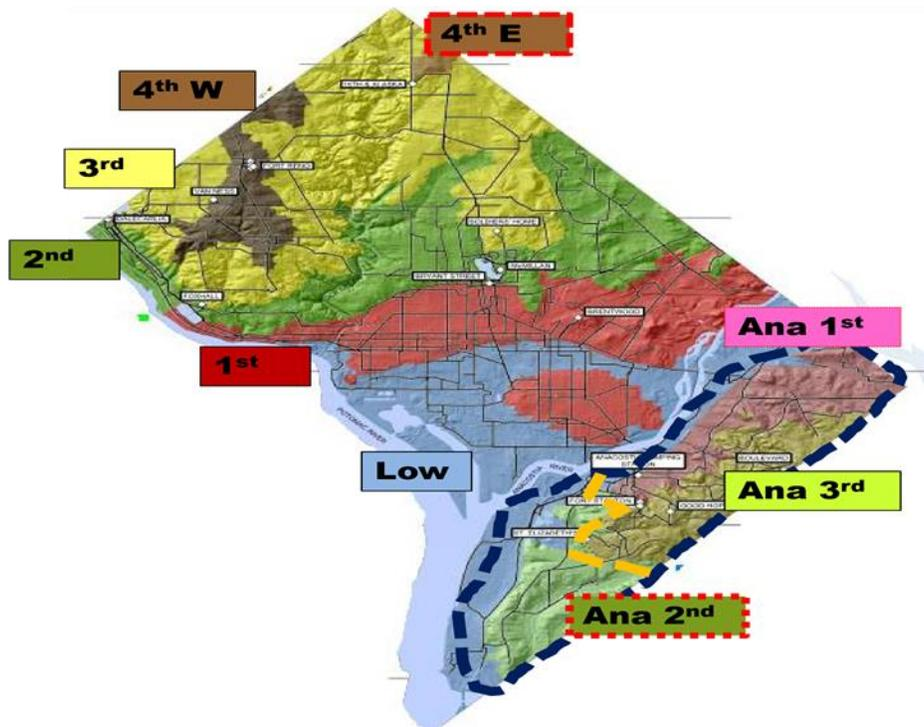
The 2<sup>nd</sup> High Service Area on average maintains a discharge pressure level in its section of the system of around 95 pounds per square inch. By contrast, the Low Service Area maintains a discharge pressure level in its section of the system of around 21-22 PSI.
