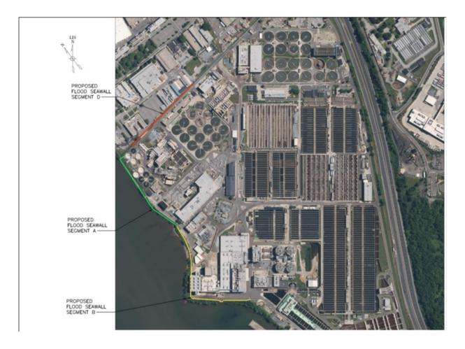
Conceptual Alignment of Floodwall Segments A, B, and D
