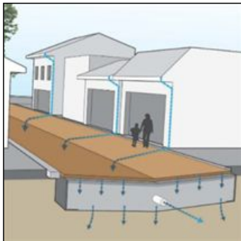
Alley Permeable Pavement (APP)
