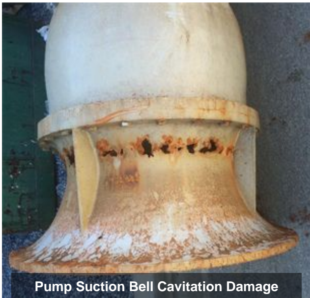
Filter Influent Pump Require Replacement
