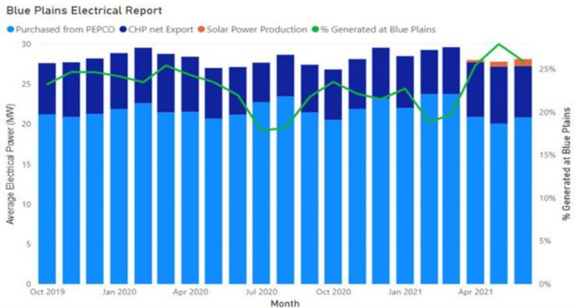
Figure 2. Blue Plains Energy Report – December 2019 to June 2021: Average Electricity Purchased from PEPCO (light blue), Net Export from CHP (dark blue), Solar Power Production (orange) and % of Total Plant Electricity Use Generated Onsite (green line on right Y-axis)
