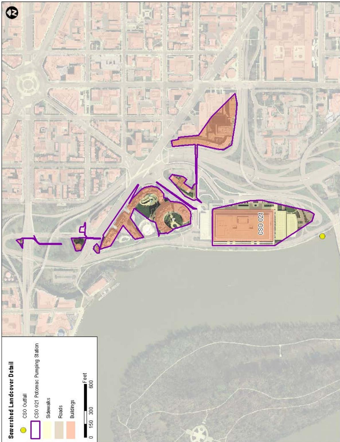
Figure A-2. Sewershed Characteristics - CSO 021, Potomac Pumping Station
