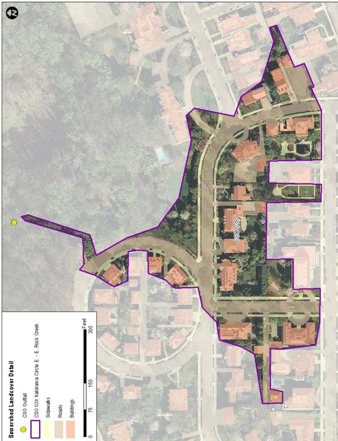
Figure A-14. Sewershed Characteristics - CSO 038, Kalorama Circle E – E. Rock Creek
