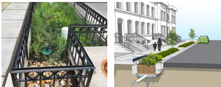
Planter Bioretention (PBR)
