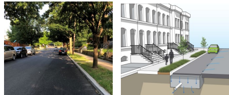
Parking Lane Permeable Pavement (PPP)
