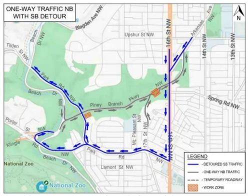
Figure 3-3. Proposed Detour Route for Partial Closure of Piney Branch Parkway NW
