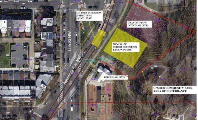
Figure D-6. Upstream Storage Tanks with Pump Station – Storage Facility 01
