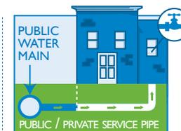
Lead can enter your water if you have a lead service pipe or household plumbing with lead. Orthophosphate can reduce lead release from these sources.
